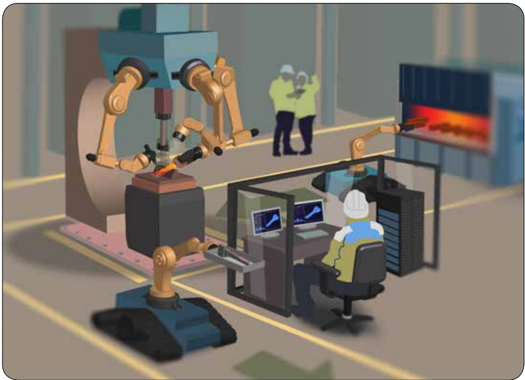
Figure 11. Conceptual metamorphic manufacturing equipment suite (containing the five fundamental elements of metamorphic manufacturing represented by the acronym STARC, and described above).
