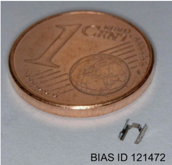
Fig. 5.20 Micro bending element (spring element from Fa. Harting GmbH & Co, Germany)
