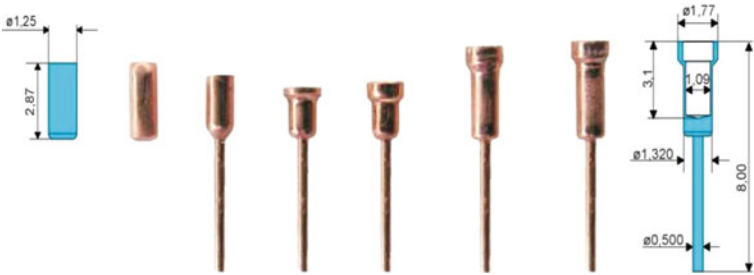
(c) direct forward / backward cup extruded copper pin (reference: Wafios GmbH)
