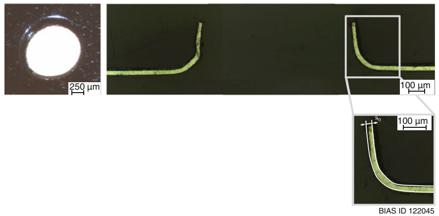
Fig. 5.29 Material: 1.4301, size25, flaring ratio 1.6, d_p = 1.0 \text{ mm} . Left Formed flange. Rim is uneven due to oxidation effects of pre-hole generation by sublimation cutting. Right cross-sectional view, V2A-etchant
