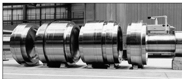
Figure 1. Assembly of forged turbine disks of different material grades for the production of a welded turbine rotor [7].
