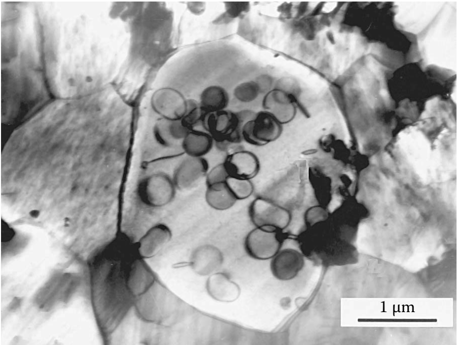
FIGURE 6.21 A typical feature of the microstructure of ultra-fine-grained Zn-Mn alloys when deformed at temperatures lower than or at a strain rate higher than the optimum for superplasticity is the appearance of vacancy loops in the grains. The appearance of point defects can be explained by insufficient diffusion flow that is unable to ensure the complete accommodation of adjacent grains. This is demonstrated in the micrograph of an ultra-fine grained Zn-0.7%Mn alloy after deformation at a deformation rate \dot{\epsilon} = 1.10^{-3} \text{ s}^{-1} at 300°C. The maximum elongation was only 60%. Note that the shape of MnZn 13 particles is not rounded but somewhat faceted and that their size is much larger than in the Zn-1.2%Mn alloy (see Figure 6.19 ). Obviously the applied temperature-strain rate interval, which was optimal for the Zn-1.2%Mn alloy, is not suitable for the lower manganese alloy to reach superplastic state.
