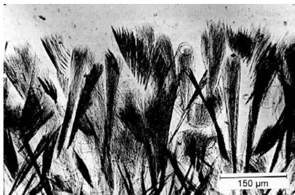
Fig. 3.9. Devitrite \text{Na}_2\text{O} \cdot 3\text{CaO} \cdot 6\text{SiO}_2 crystals in a soda-lime-silicate glass having the characteristic shape of a shavingle-brush [539]
