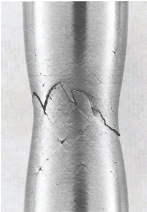
Fig. 3 Low-carbon cast steel test specimen emphasizing 45° shear aspect of tensile fracture of a ductile metal. Diagonal ridges are “Lüders lines” or “stretcher strains”; porosity in the steel shows many localized fractures.
