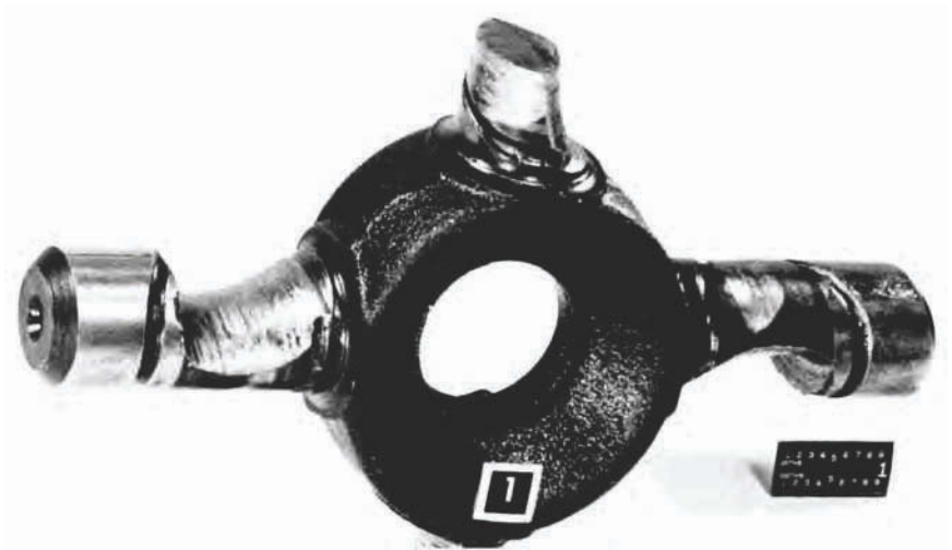
Fig. 12 Destructive adhesive wear of a differential cross following fracture of one severely worn trunnion. This vehicle was operated primarily in forward speeds; consequently, only the forward-drive side was damaged severely by the rotation of differential pinions on the trunnions. The lubricant was inadequate for this application. The differential cross, or spider, and the differential pinions were made of carburized and hardened steel.
