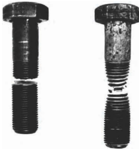
Fig. 1 Brittle versus ductile fracture in two 1038 steel bolts deliberately heat treated to have greatly different properties when pulled in tension. The brittle bolt (left) was water quenched with a hardness of 47 HRC but had no obvious deformation. The ductile bolt (right) was annealed to a hardness of 95 HRB (less than 20 HRC) and shows tremendous permanent deformation.
