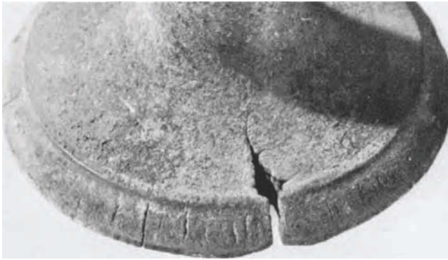
Fig. 8 Thermal-fatigue crack in the hardfacing alloy on an exhaust valve from a heavy-duty gasoline engine ( \sim 2.5\times ). Advanced burning originated from the large crack. Additional thermal-fatigue cracks are also present on the valve face. Engine efficiency rapidly deteriorates from increasing loss of compression when very hot exhaust gases blast through the open passage (also called blowby ).
