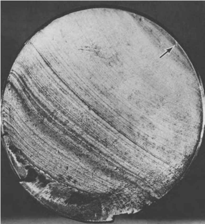
Fig. 24 Large axle shaft of medium-carbon steel with fatigue fracture across most of the cross section before final rupture. Note the smooth origin region (arrow) and gradually coarsening fracture surface as the fatigue crack progressed. Note that there was a thread groove running around the periphery and that the fracture origin is in the root of the thread. However, the nominal stress was quite low because the part was still intact and operating even though the fatigue crack had gone nearly all the way through the section. This indicates that only a slight improvement in the thread groove would be necessary to prevent this type of long-term fracture.
