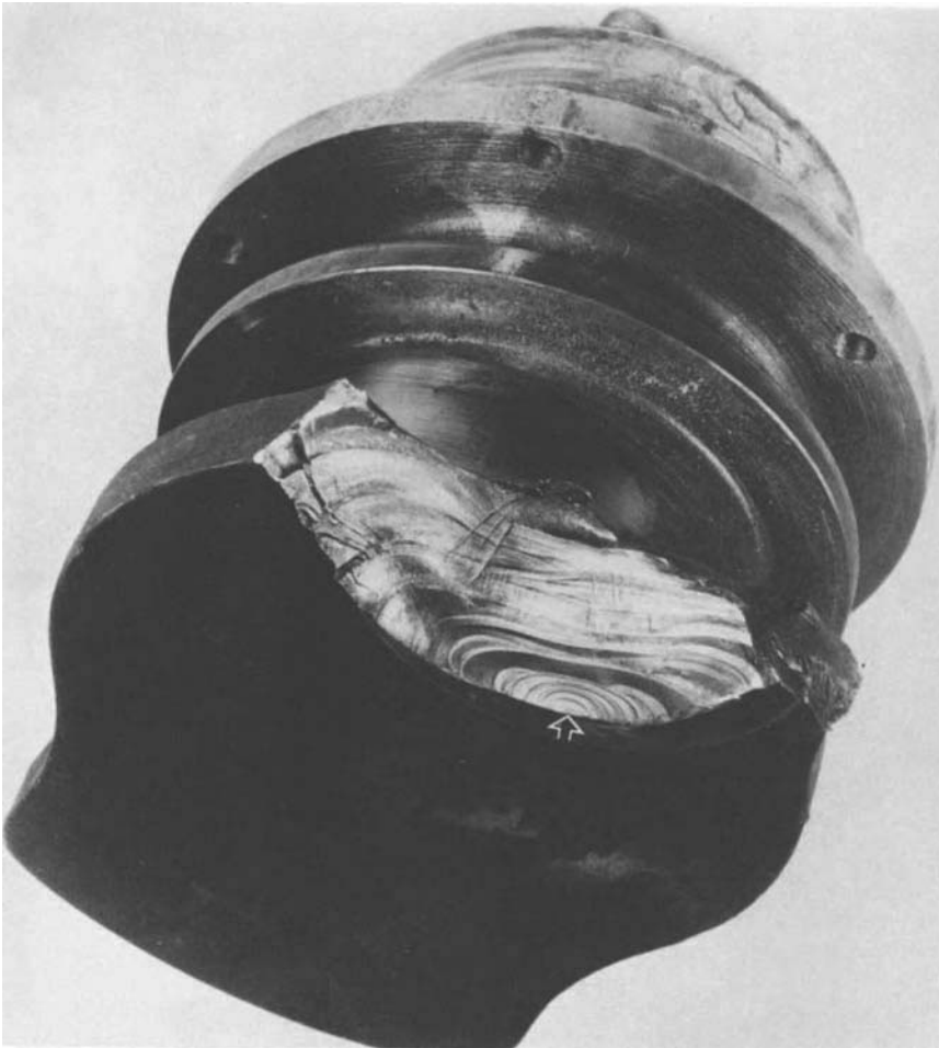
Fig. 32 Bending fatigue fracture through the cheek of a diesel engine crankshaft. The very prominent steps and beach marks were the result of severe overloading during starting and clutching with a very aggressive friction material in the clutch. Though this was a laboratory test, it was not operated continuously and thus more closely resembles fracture from actual vehicle service.
