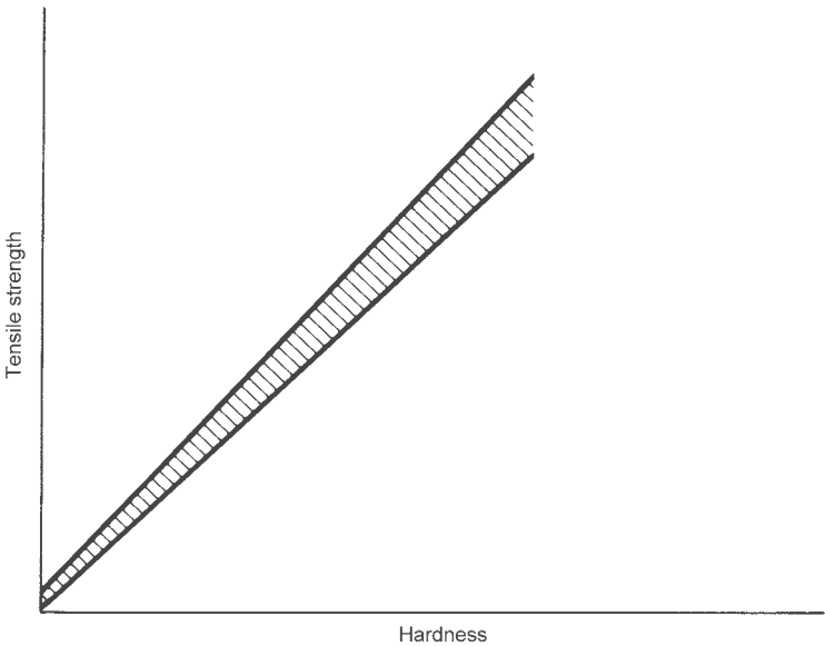
Fig. 8 Relationship between hardness and tensile strength of metals in the absence of stress concentrations
