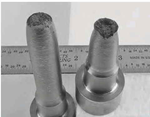
Fig. 2 A fractured tensile specimen with the typical cup-and-cone fracture characteristic of ductile metals fractured in tension.
