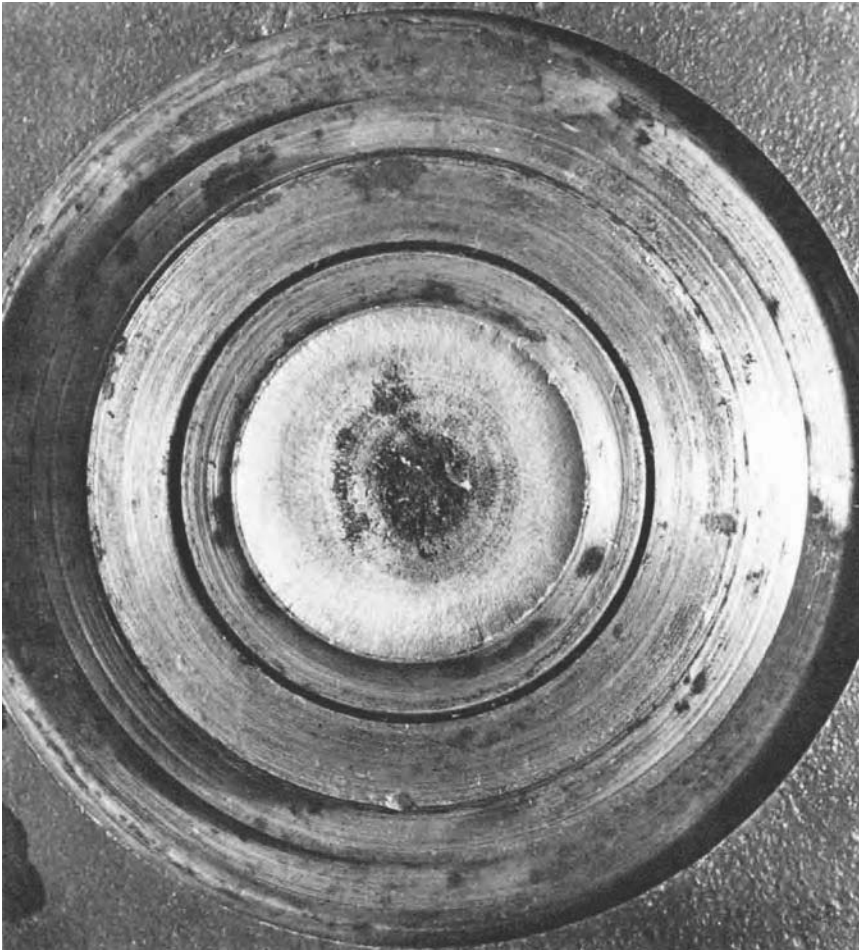
Fig. 30 Rotating bending fatigue fracture of a 2-in.-diam grade 1035 steel shaft, hardness 143 HB. The part was designed with a large radius joining the shaft to the shoulder, but it was machined with a sharp tool mark in the fillet. Multiple-origin fatigue around the periphery proceeded uniformly into the shaft, finally fracturing with a final rupture region in the center of the shaft.
