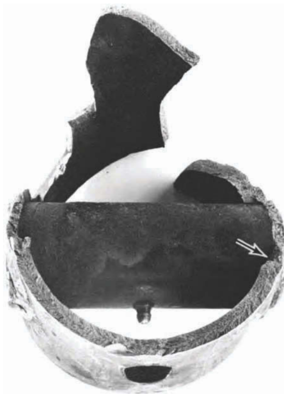
Fig. 7 Surface of a brittle fracture in a cold-drawn, stress-relieved 1035 steel axle tube. Fracture originated at a weld defect (arrow) during testing in very cold weather. Note the well-defined chevron marks located clockwise from the arrow, pointing back toward the origin. Note also that the steel around the access hole below the grease fitting is actually necked down along the tube axis. The upper side of the tube is deformed and torn in a ductile manner.
