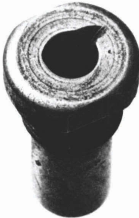
Fig. 3 Abrasive wear of a yarn eyelet made of hardened and tempered 1095 steel. Grooving was caused by a sharp change in direction of the yarn as it came out of the hole. Service life was improved by changing the eyelet material to M2 high-speed tool steel, which contains spheroidal carbides in a matrix of martensite. Service life probably could have been improved also by changing the angle of exit or by rounding the corner to make a bell-mouth hole. Source: Ref 1
