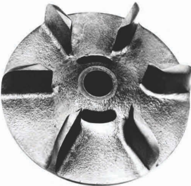
Fig. 4 Erosive wear of a gray cast iron water pump impeller. The sharp corners of the (a) new impeller have been (b) completely rounded off by the abrasive wear of sand in the cooling system. The change in shape of the vanes reduces the efficiency of the pump; if abrasive wear were to continue long enough, the vanes—and efficiency—would be completely gone.
