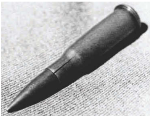
Fig. 6 Stress-corrosion crack in thin neck of a cartridge case
