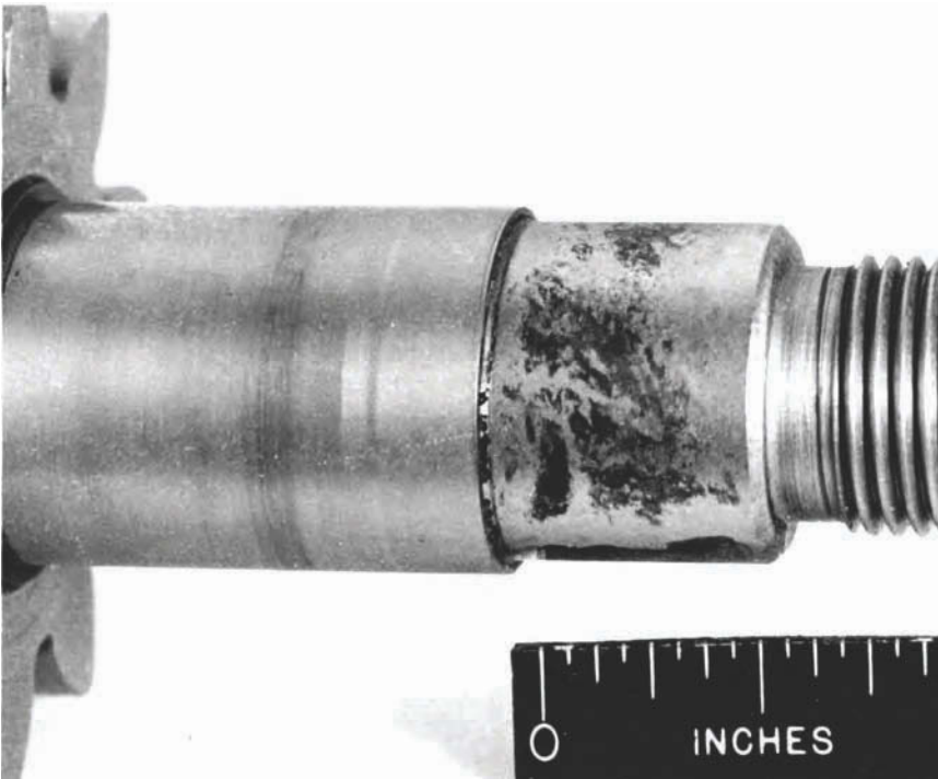
Fig. 13 Fretting wear on a steel shaft at the interface with the hub intended to be a press fit ( \sim 2.5\times ). The same fretting also appeared on the bore of the hub. This is typical of damage in a joint that is nominally stationary but in reality has slight movement between the hub and the shaft.
