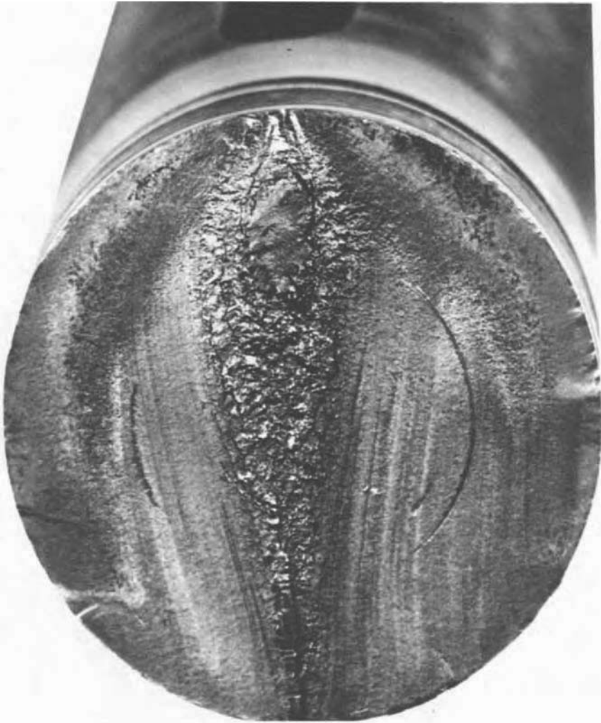
Fig. 26 Reversed bending fatigue of a 1.6-in.-diam shaft of 1046 steel with a hardness of approximately 30 HRC. Note the symmetrical fatigue pattern of beach marks on each side, with the final rupture on the diameter. This indicates that each side of the shaft was subjected to the same maximum stress and to the same number of load applications. The C-shaped marks are postfracture damage.
