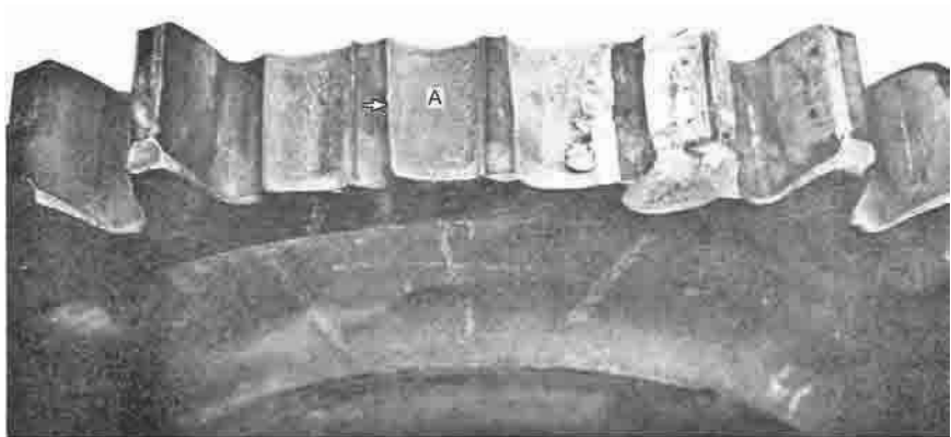
Fig. 40 Bending fatigue fractures in several teeth of a grade 8620 steel spur gear, carburized and hardened to 60 HRC in the case. It can be seen that tooth A fractured first, for it has the largest fatigue area, originating in the fillet on the arrow side of the tooth. Gear teeth are carefully shaped cantilever beams and can be diagnosed in this way. Fracture of the first tooth caused abnormal loading on the adjacent teeth, and they also rapidly fatigued, for the mating gear did not now mesh properly with them. Considerable smashing and battering of adjacent teeth is normal after gear-tooth fracture.
