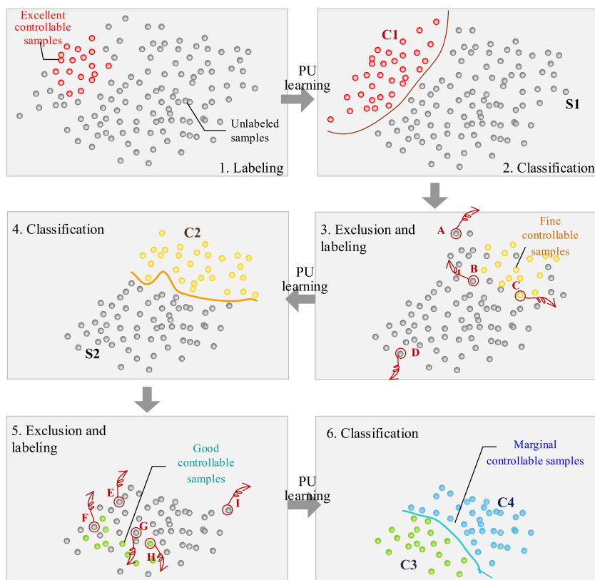
FIGURE 5.4 The procedure of controllable domain classification based on kNN-PU learning (A to I are the rejected irrational-operated samples, S1 and S2 are the first and second left sample sets, respectively, and C1, C2, C3, and C4 are the excellent, fine, good, and marginal controllable sample sets, respectively).
