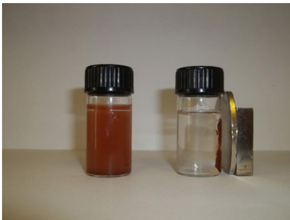
Fig. 7.8 Disperse \text{ZnFe}_2\text{O}_4 nanoparticles and their separation from solution via the application of a magnetic field (Adapted from [30] with permission from Elsevier)
