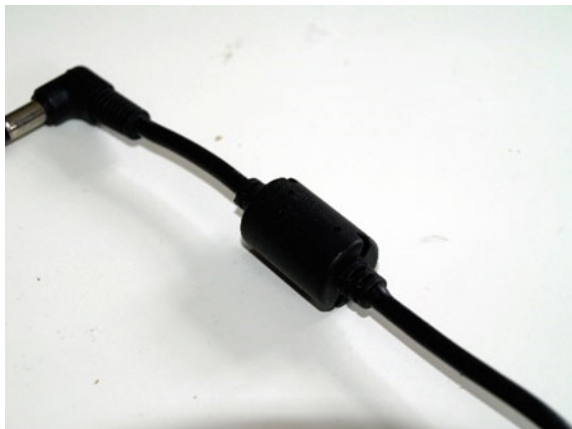
Fig. 7.3 Ferrite bead on a computer power cable (Source “Ferrite bead” by Santeri Viinamäki licensed under CC BY-SA 4.0)
