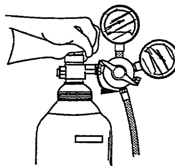
Fig. 61. Release the pressure adjusting screw by turning counterclockwise before opening the cylinder valve. Stand to one side when opening the cylinder valve.
