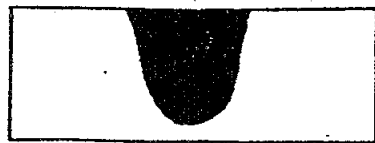
DC Electrode negative — deep penetration narrow weld
