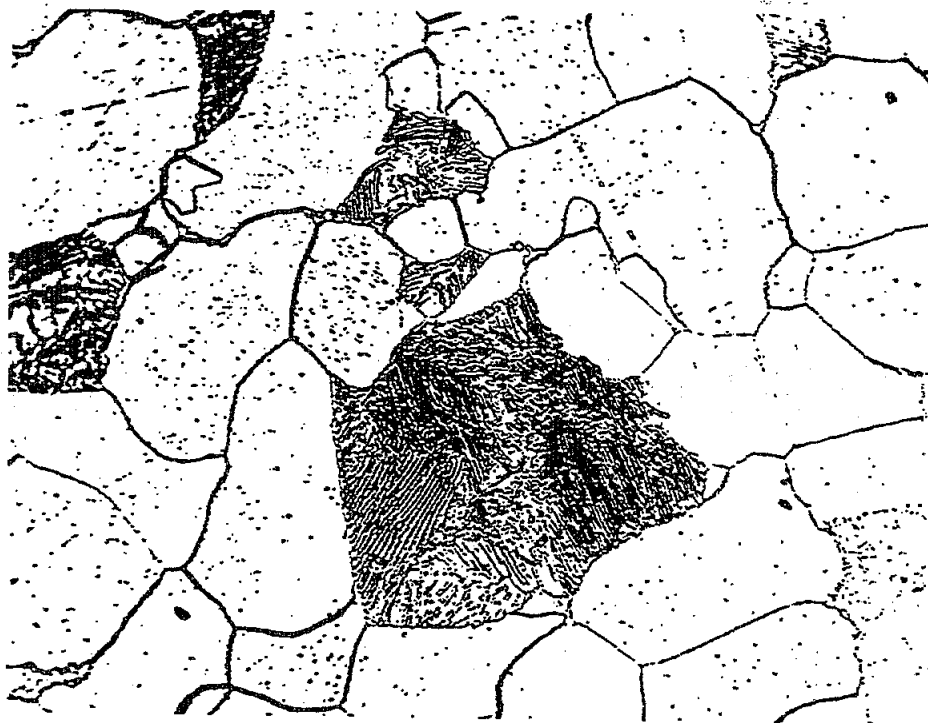
Figure 21. Structure of a typical 0.15% carbon steel cooled slowly (magnification X 1000).
