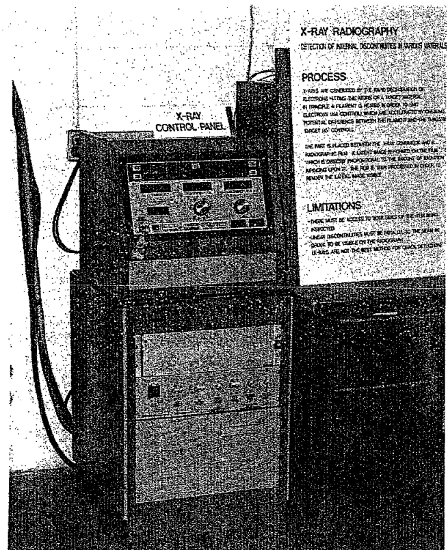
Figure 4. X-ray unit showing tube head and control panel.
