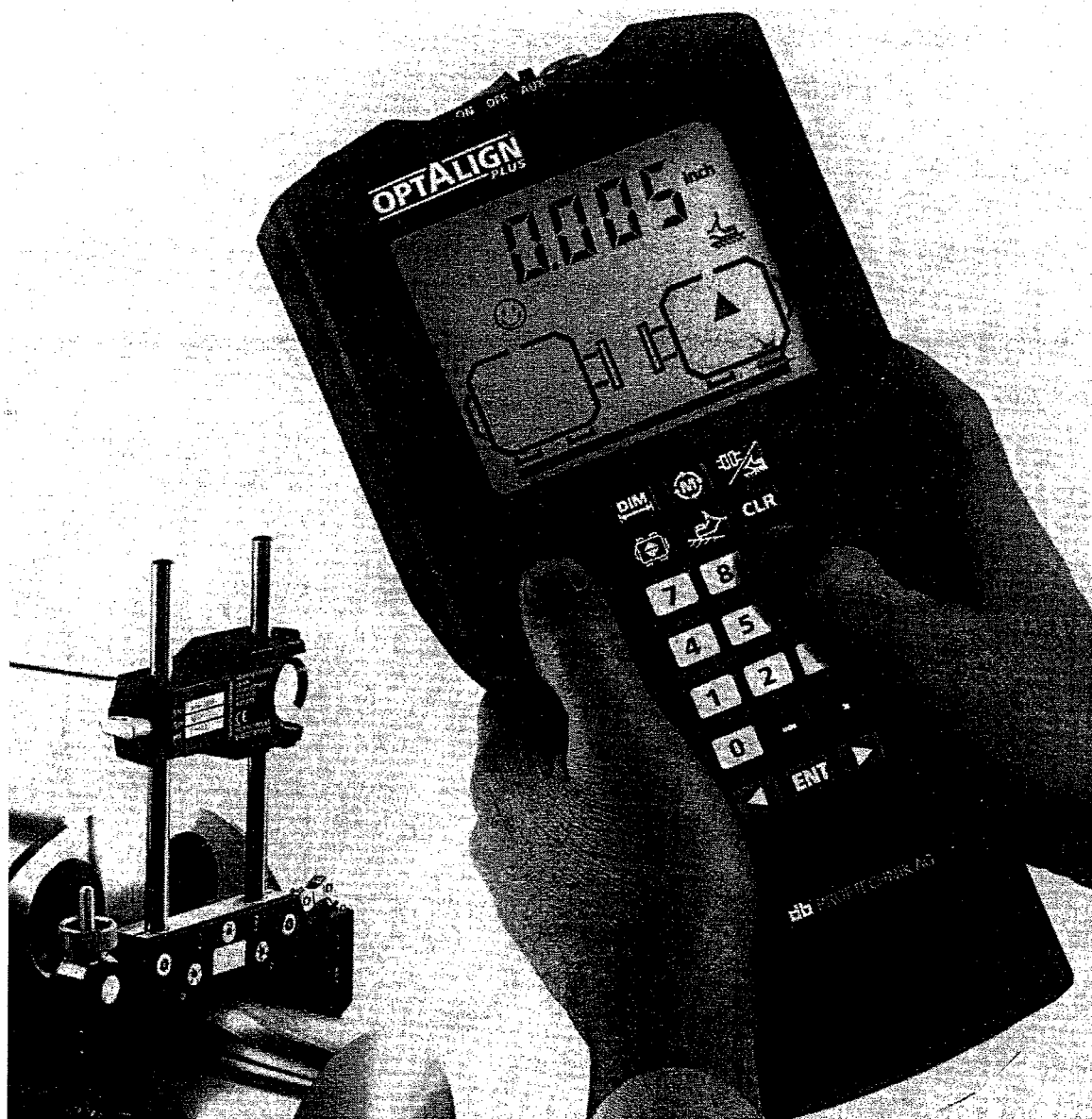
Figure 5-11. Optalign® laser-optic alignment system.
