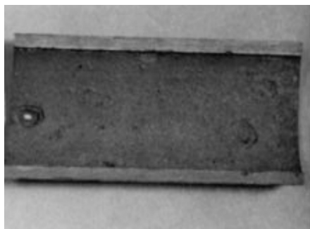
FIGURE 18: Oxygen Attack Occurs as a Distinctive Pit Formation
