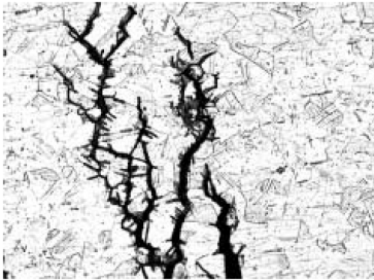
Figure A7: Photomicrograph of Caustic SCC in UNS S32100—Magnification 500X
