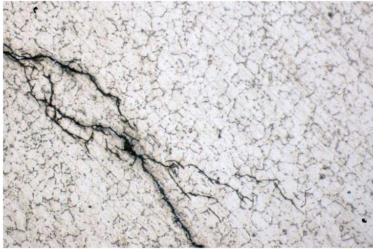
Figure A11: Photomicrograph of Caustic SCC in UNS N08825—Magnification 200X
