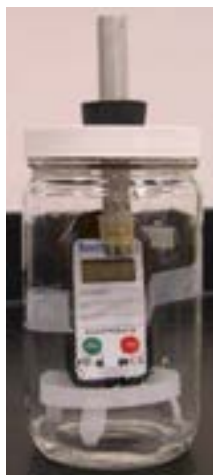
Figure 3a: Datalogger Inside the Jar-Test Apparatus, Held with Low-Acid Transparent Adhesive Tape
