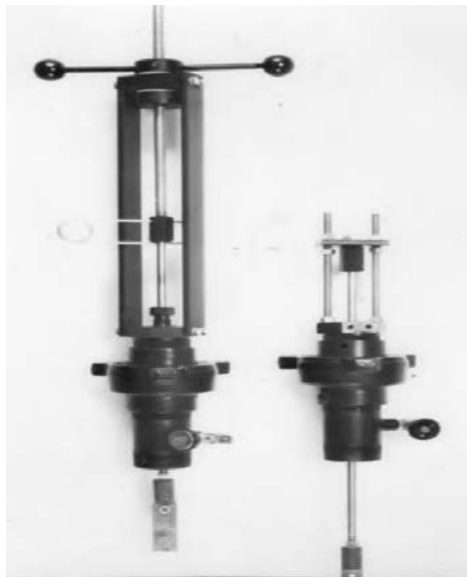
Figure 5: Tool for Installing and Removing Coupons in Systems under Pressure. The Pipe Nipple Screws into an Existing Valve on the Line or Vessel. Complete Assembly is Shown on Left. After the Coupon has been Positioned, the Drive Unit is Removed and the Coupon Holder is Locked as Shown on the Right
