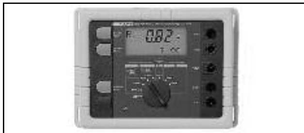
Figure 33. Example of an earth ground resistance tester
