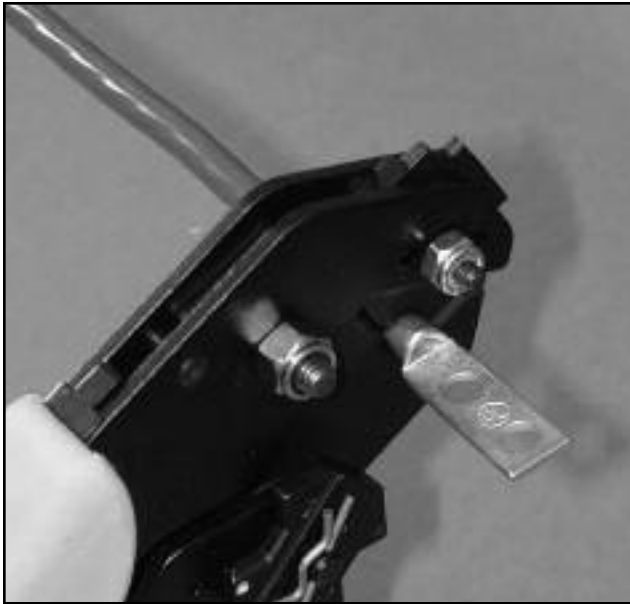
Figure 13. Example of crimping a conductor in the barrel of the lug
