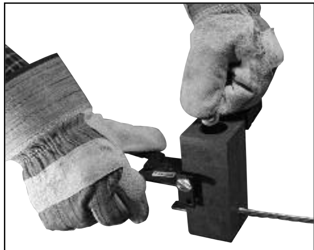
Figure 16. Mold being locked and disk inserted
