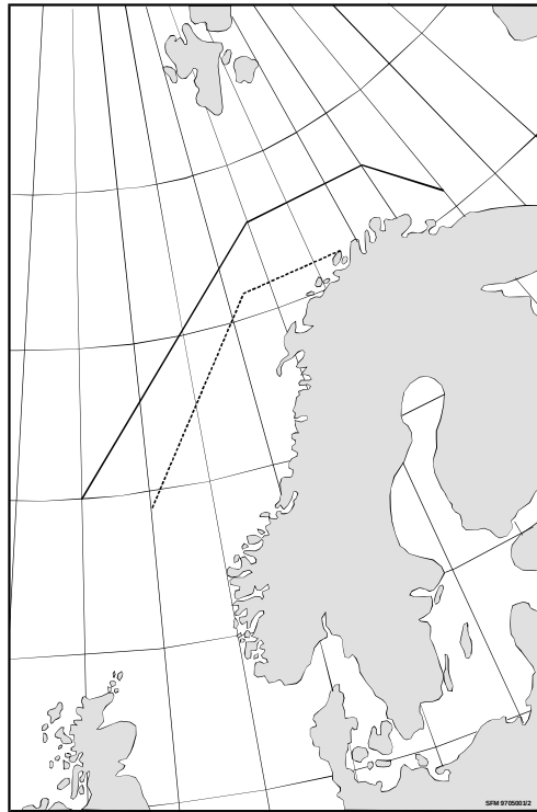
Fig. 6.4.1 Limit of sea ice in the Barents Sea with annual probability of exceedance of 10^{-2} (solid line) and 10^{-4} (dotted line).
