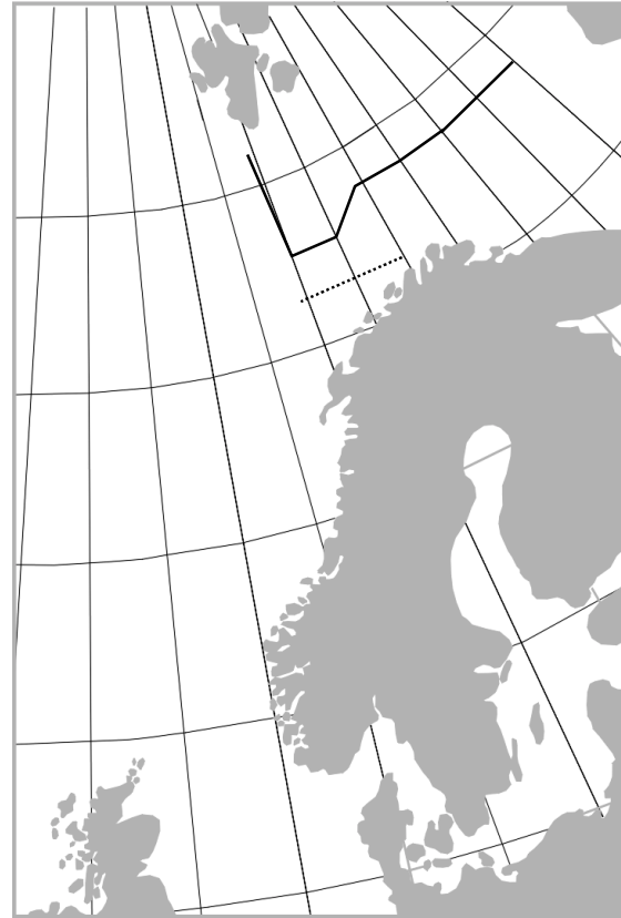
Fig. 6.4.2 Limit for collision with icebergs with a probability of exceedance of 10^{-2} (solid line) and 10^{-4} (dotted line)
