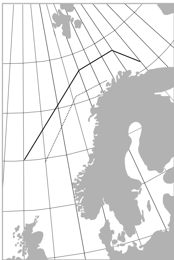
Figure 5 - Limits of sea ice in the Barents Sea with annual probability of exceedance of 10^{-2} (solid line) and 10^{-4} (dotted line)
