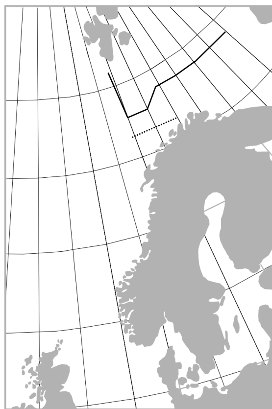
Figure 6 - Limit for collision with icebergs with a probability of exceedance of 10^{-2} (solid line) and 10^{-4} (dotted line)
