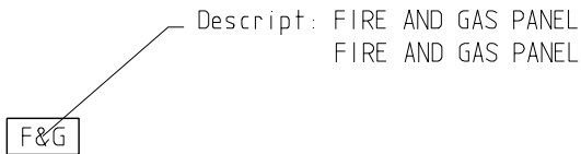
SF019A FIRE AND GAS PANEL
