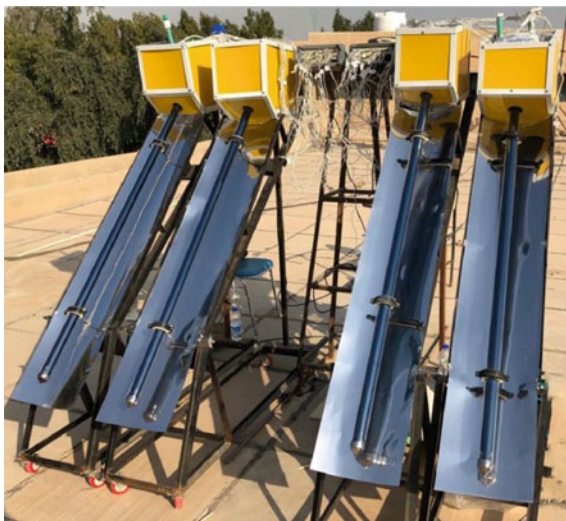
Fig. 1 Experimental setup of evacuated tube solar water heater by Alshukri et al. [20]. Copyright Elsevier {Lic # 5510340802537}
