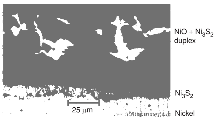
Figure 7.13 Optical micrograph of a duplex scale formed on nickel heated to 500°C in Ar-1% SO 2 .
