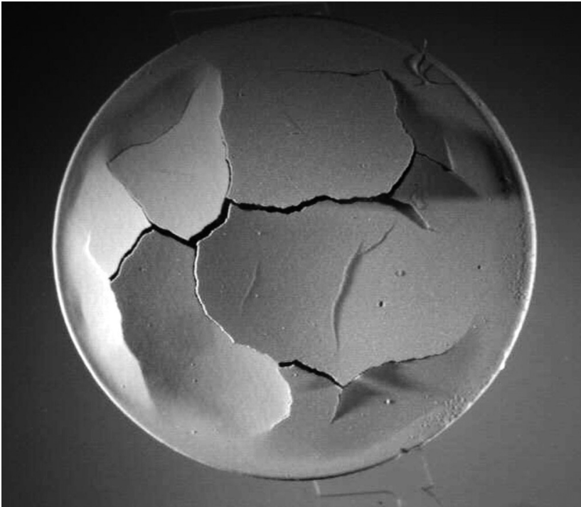
Figure 10.24 Optical micrographs showing the failures of an EB-PVD topcoat with a Pt-modified aluminide bond coat. See text for details.
