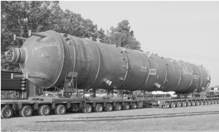
8.3 Stainless steel clad refinery column. 4.6 m ID × 35.3 m long × (100 mm Cr–Mo steel + 3 mm type 321 stainless steel).
