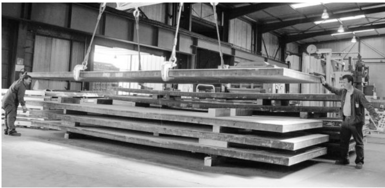
8.2 Titanium-steel EXW clad plates being prepared for shipment, 2100 mm × 8000 mm × (125 mm steel + 8 mm titanium Gr 17).
