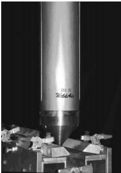
7.15 Photograph of the ISF-non-vacuum nozzle system.
