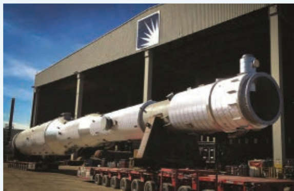
▲ This 150-ft demethanizing tower exceeding 300 tons is an example of Spitzer's complex manufacturing capabilities.
