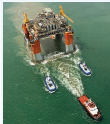
▲ The OPTI® semisubmersible hull is scalable to meet operator needs and is water depth independent. OPTI-EX® installed July 2011 (shown left), and Delta House installed September 2014 (shown right).
