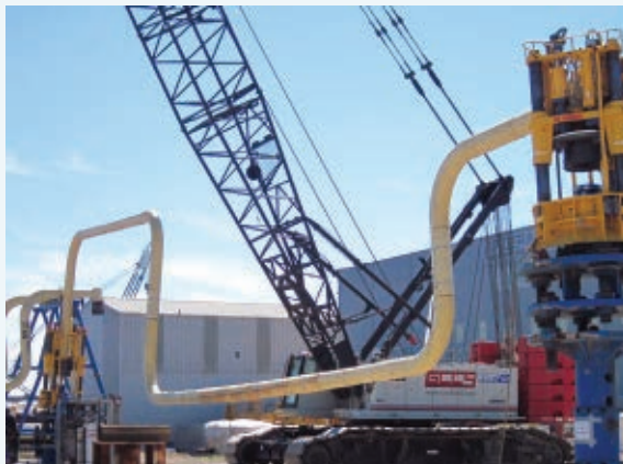
▲ Jumper with Auto-Therm® GSPU Insulation.
