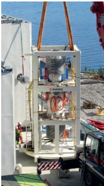
The OneSubsea Multiphase Compressor enables a very compact and cost-effective subsea infrastructure.
