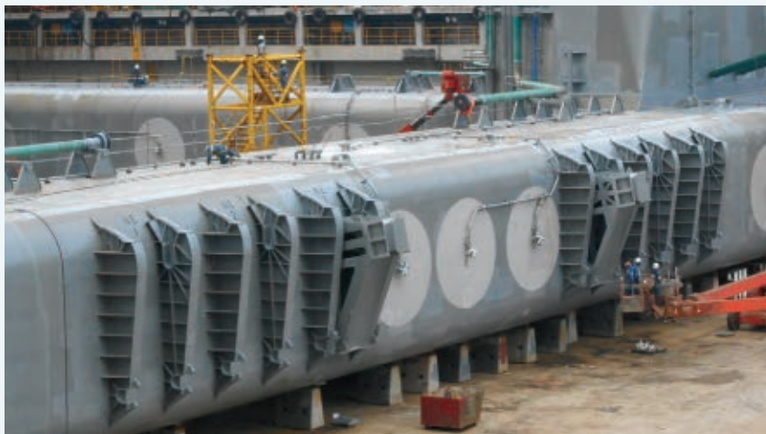
▲ The Exmar proprietary riser porch and adapter arrangement on Delta House can connect 18 risers.
