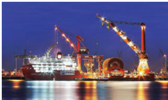
Lewek Constellation during its 800-metric ton Huisman multi-lay system installation at the Huisman Equipment quayside facility. (Photo courtesy Huisman Equipment)
