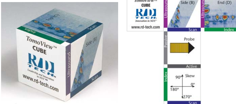
Figure 4-31 R/D Tech TomoView™ Cube (left), and showing all faces (right).
