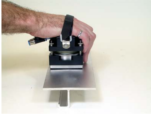
Figure 5-117 Normal beam scan of aluminum laser weld with water box.
