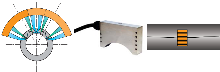
Figure 5-87 Phased array inspection of ERW pipes: principle, probe, and weld wander.
