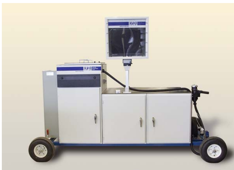
Figure 5-24 Phased array system including two QuickScan PA units.
