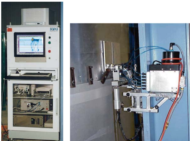
Figure 5-17 Tomoscan FOCUS 32:128, MCDU-02 driver, and computer enclosed in an air-conditioned cabinet ( left ); water recirculation system ( right ).
