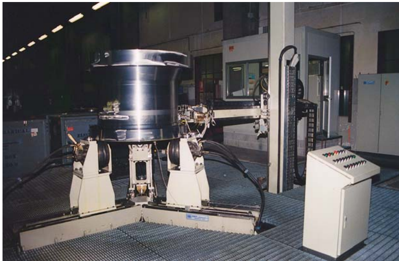
Figure 5-97 Photo of circular forging being inspected by phased arrays.
