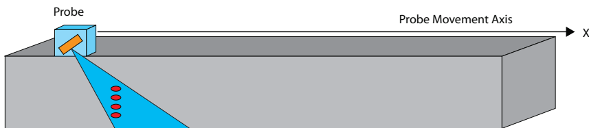
Figure 4-2 Linear scan pattern for probe characterization.
