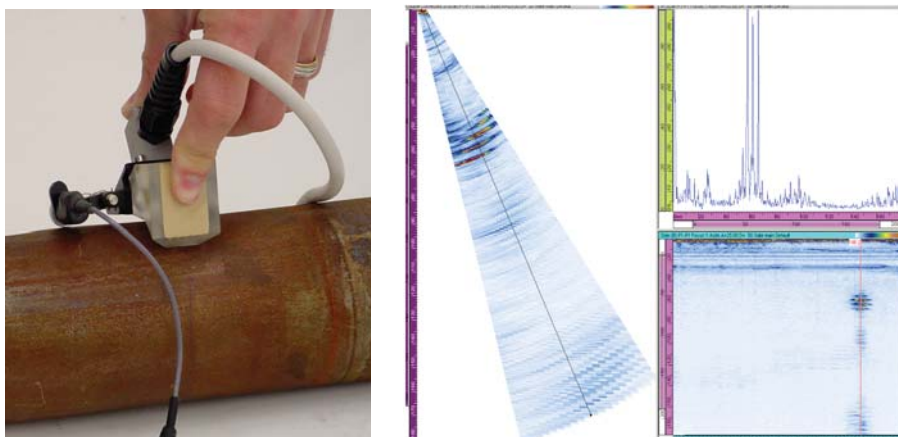
Figure 5-40 Phased array detection of fatigue cracks in CANDU® feeder tubes: scanning setup ( left ) and crack detection ( right ).
