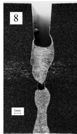
Figure A7-7. The set-up and cross-section of testpiece 7. in the TAGUCHI experiments for the first filling pass with hybrid welding. Parameters in Appendix 4.
