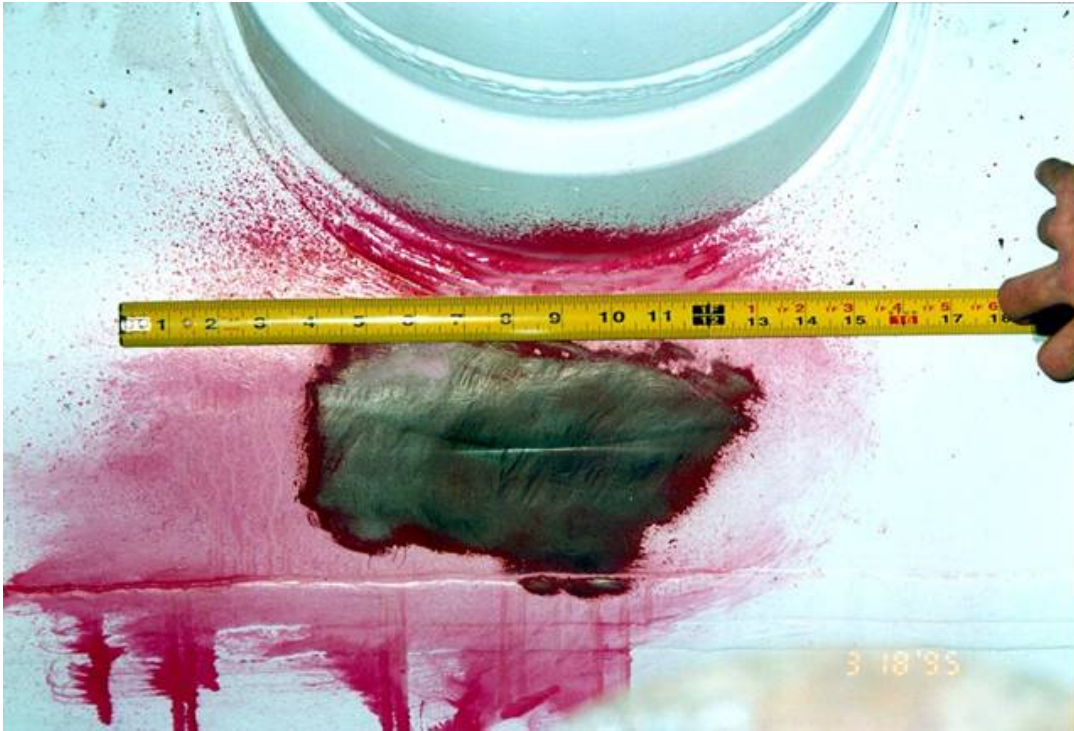
Figure 13 – Bottle Shell Crack Due to Design Fault
