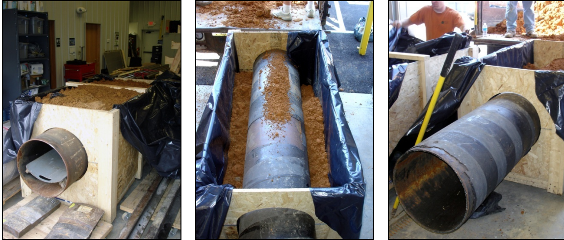
Figure 4-16. Photographs of soil box built for soil loading tests. The 20 in. coal-tar wrapped pipe used in previous studies was buried.
