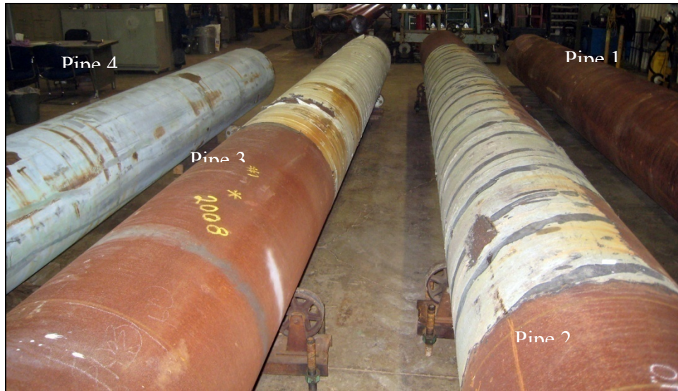
Figure 6-1. Photograph showing four pipes used for pull testing at the PSF.
