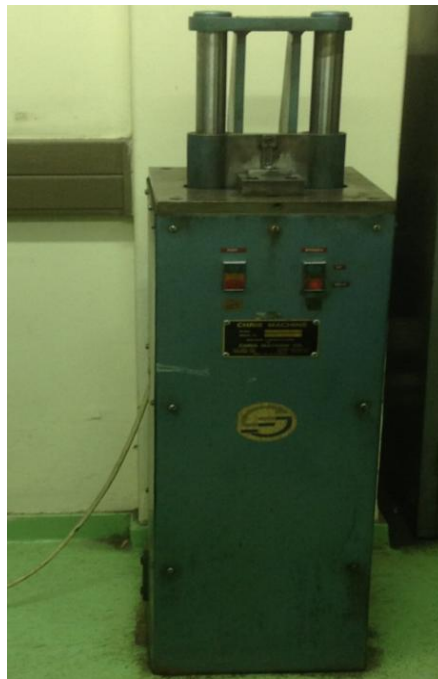
Figure 16: Chris notching machine model number SRC-CH 1B and SN: 55/300/19 that was used to notch the samples
