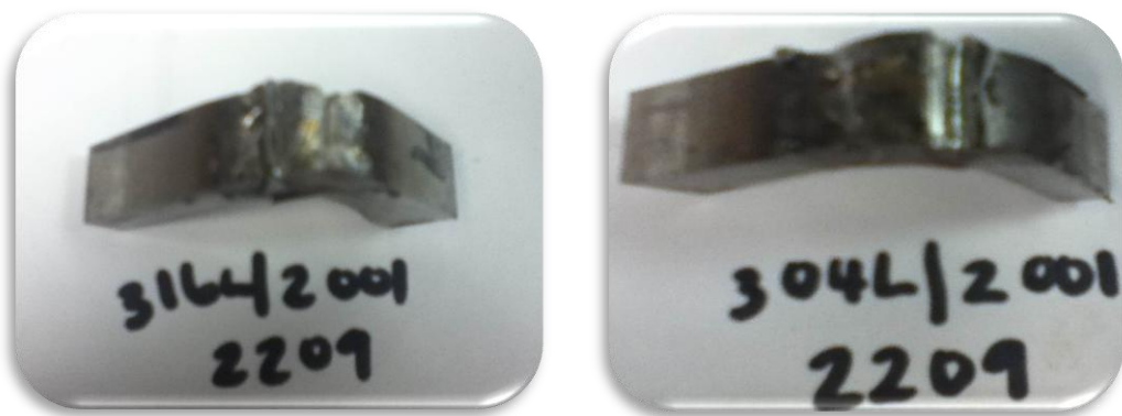
Figure 21: Photographs of impact samples welded using 2209 duplex stainless steel
