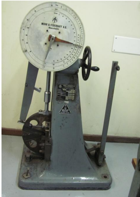
Figure 18: The Mohr and Federhaff AG, pendulum impact test machine, machine number 1046 type PSW30 that was used during the test
