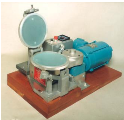
The Hoover Automatic Muller provides a quick and easy method for preparing a small sample of pigment-resin dispersion. Glass plates that shear the pigment into the resin are easily cleaned by the solvent used in solubilizing the resin. This piece of equipment continues to find new uses wherever incoming pigment quality is a concern.
