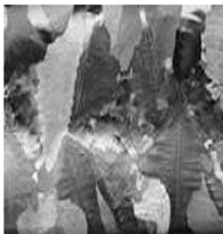
Fig 16.11 Microstructure of pure aluminium
