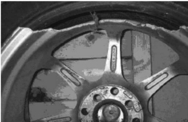
Fig. 8.1 Fatigue fracture of the rim of a car wheel
