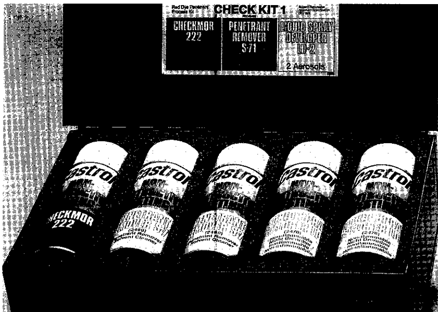
Fig. 7.1 Field test kits: the flexibility of the penetrant method of NDT allows the apparatus to be reduced to a portable case of aerosol cans.
