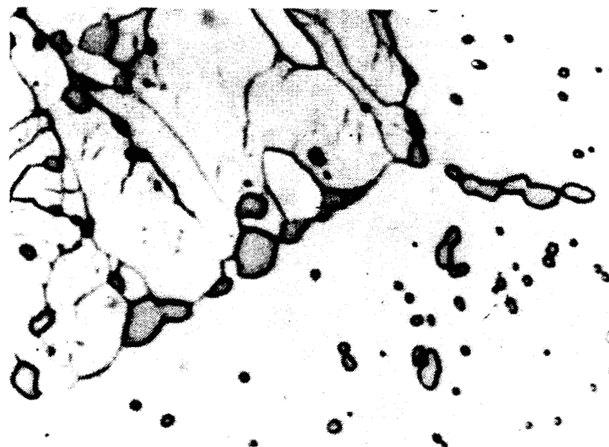
Fig. 6.32 A partially recrystallized structure. Top left: recovered but not recrystallized, bottom left: a new recrystallized grain. Coarse spheroidal cementite is also apparent. Fe-0.18 C quenched and tempered 96 h at 600 °C ( \times 2000 ). (After G.R. Speich, in Metals Handbook , 8th edn., Vol. 8, American Society for Metals, 1973, p. 202.)
