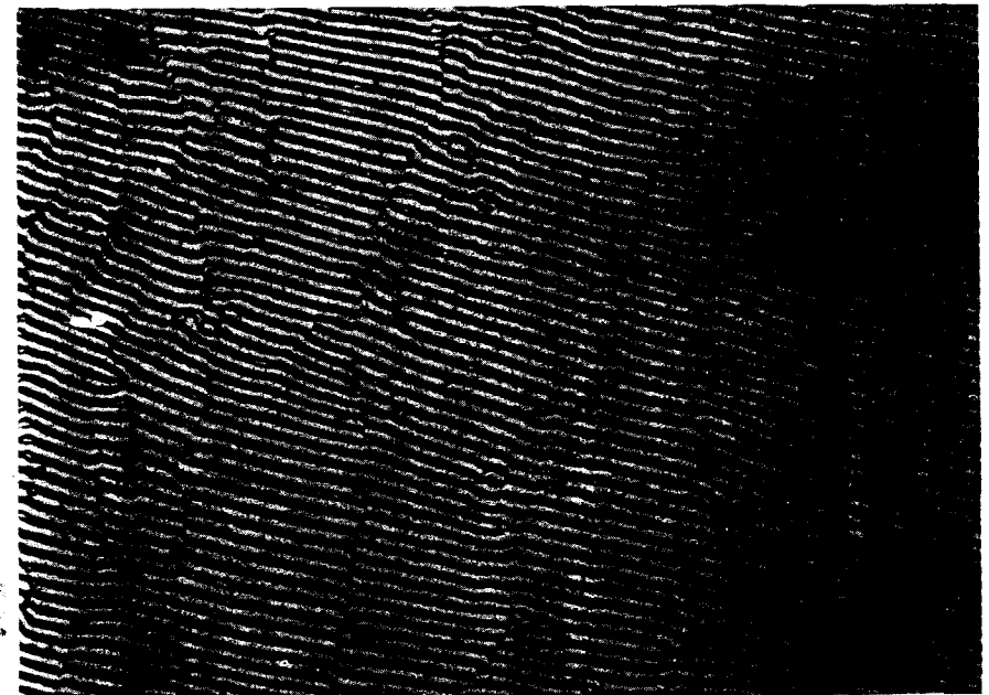
Fig. 4.29 Al-Cu \text{Al}_2 lamellar eutectic normal to the growth direction ( \times 680 ). (Courtesy of J. Strid, University of Luleå, Sweden.)
