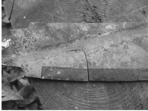
FIGURE 15.2 A quench crack extending from the surface to the core. 2
