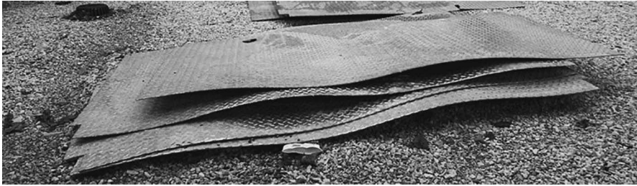
FIGURE 15.1 Warping steel plates due to galvanization. 1
