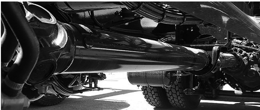
FIGURE 16.2 Driveshafts as used in automobile applications. 2
