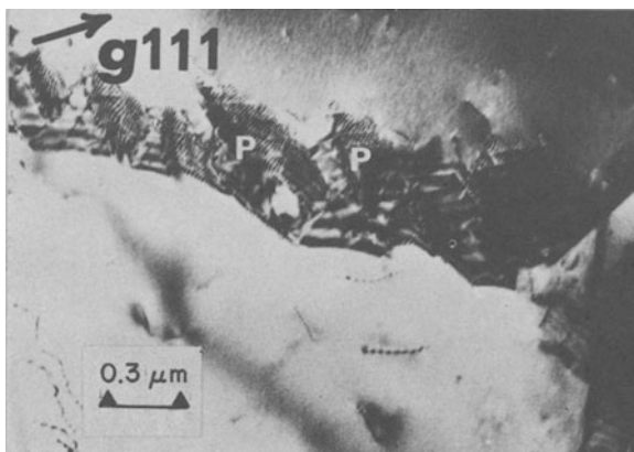
Figure 4.28 BF image of Cr 23 C 6 precipitates in an austenitic stainless steel direct quenched from 1050 °C and aged at 700 °C for 30 min [Courtesy of P. H. Pumphrey]
