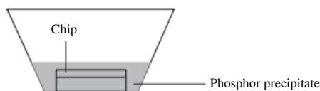
Fig. 6.22. Profile of fluorescent powder dried in solution.
