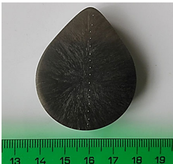
Fig. 10.61 Macrography of the cam F
