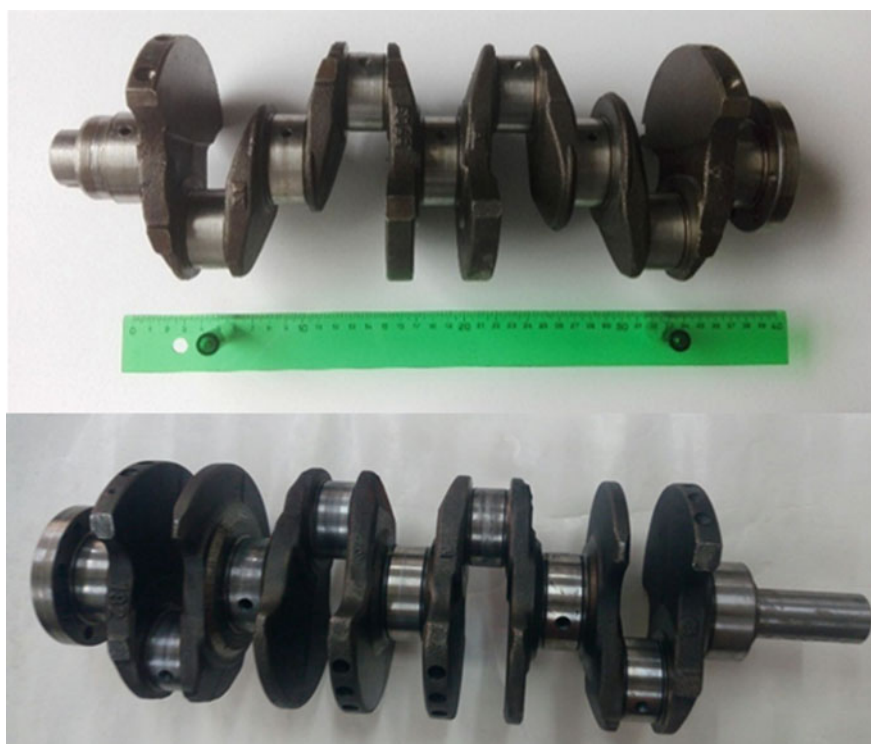
Fig. 10.71 Macrography of a crankshaft (steel, upper; ductile iron, lower)
