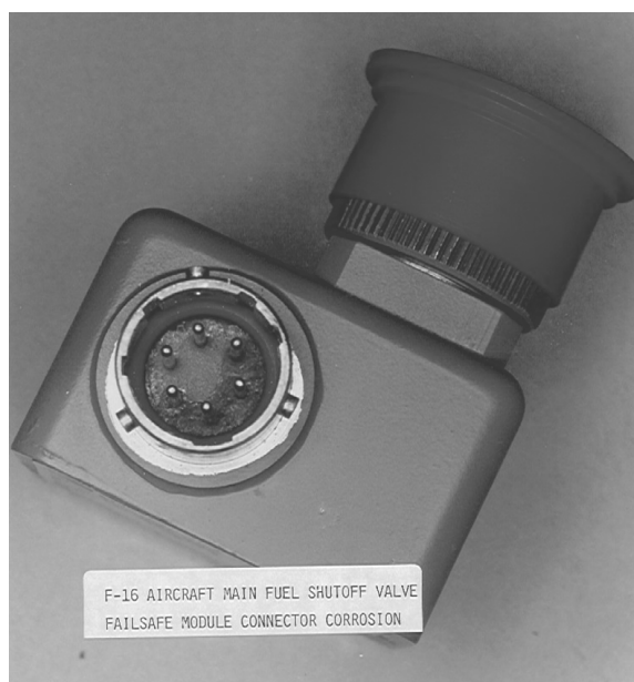
Fig. 2.2 Tin-plated pin corrosion in failsafe module connector on F-16 actuator found in the closed position with master fuel switch to master. (Courtesy David H. Horne, Hill AFB, Utah.)
