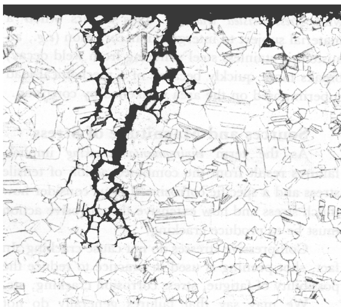
Fig. 2.23 Typical intergranular stress corrosion cracks in cartridge brass (70 Cu, 30 Zn). Etched 30% \text{H}_2\text{O}_2 , 30% \text{NH}_4\text{OH} , 40% \text{H}_2\text{O} . X75. (Corrosion Basics: An Introduction, 2nd edition, NACE International, by permission.)
