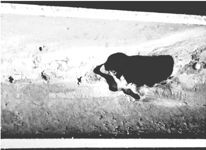
Fig. 2.19 Erosion–corrosion of a brass tube carrying out seawater. (Courtesy Defence R&D Canada-Atlantic.)
