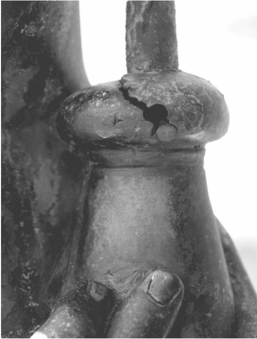
Fig. 2.25 Stress corrosion crack in a bronze monument caused by build-up of rust around a decorative steel rod. (Courtesy Kingston Technical Software.)
