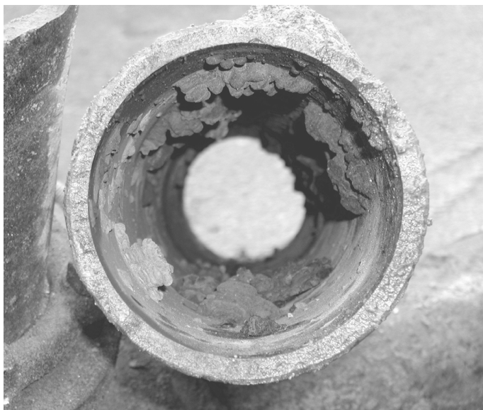
Fig. 3.32. Tubercles in a small diameter water pipe. (Courtesy Public Works and Services, City of Ottawa.).
