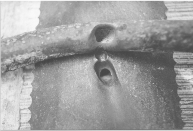
Fig. 2.4 Pits in the galvanized water pipe that contributed to the erosion corrosion of the gas line and the subsequent leak in a sewer main that caused the Guadalajara 1992 explosion (7). (Courtesy of Dr. Jose M. Malo, Electric Research Institute, Mexico.)
