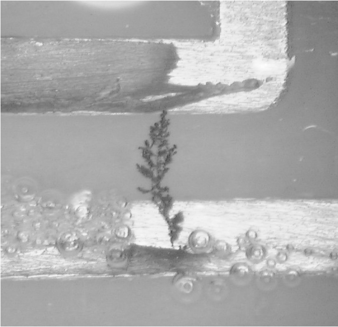
Fig. 2.3 Dendrite on a circuit board after its exposure in a test chamber. (Courtesy David A. Douthitt LoCanLLC.)
