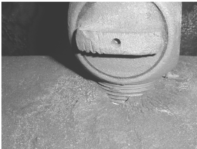
Fig. 2.16 Corrosion of a water main ductile iron adjacent to a copper fitting. (Courtesy Public Works and Services, City of Ottawa.)
