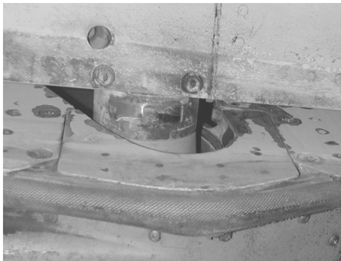
Fig. 2.20 Fretting corrosion at the interface of two highly loaded surfaces that are not designed to move against each other. (Courtesy Mike Dahlager Pacific Corrosion Control Corp.)
