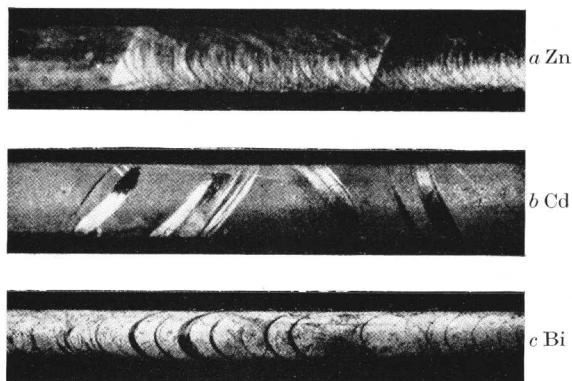
FIG. 48 (a)–(c).—Mechanical Twinning of Metal Crystals.
