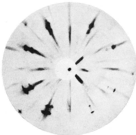
(b) Al crystal extended at elevated temperature; 4-fold picture: T = (001); (11\bar{1}) .
