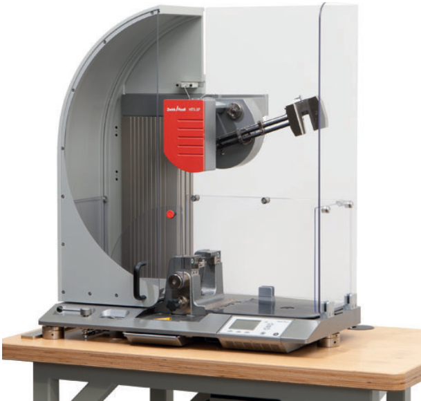
CHARPY IMPACT TEST Pendulum impacts on test bar
