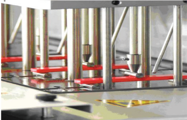
Figure 10.10 HDT machine test detail; source: Zwick-Roell
