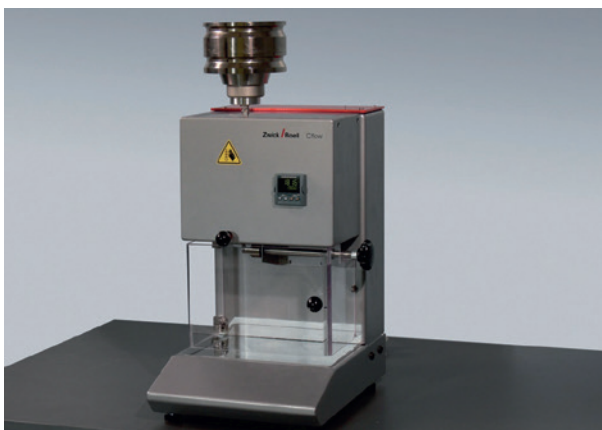
Figure 10.2 Plastometer to determine melt mass flow rate; source: Zwick-Roell
