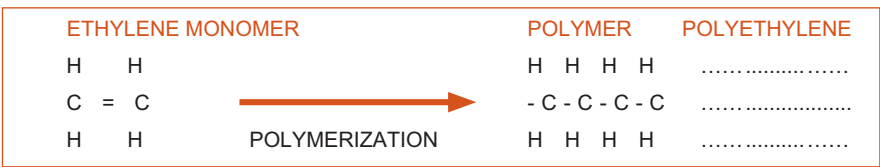
Figure 1.1 Example: ethylene monomer (molecule)
