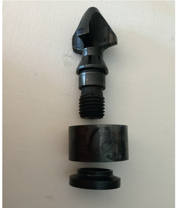
Figure 13.16 Non-return valve parts: ring closure, seat ring, and screw tip
