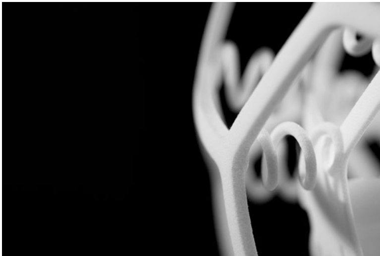
Fig. 5.1 Advanced functional geometry created via polymeric laser sintering
