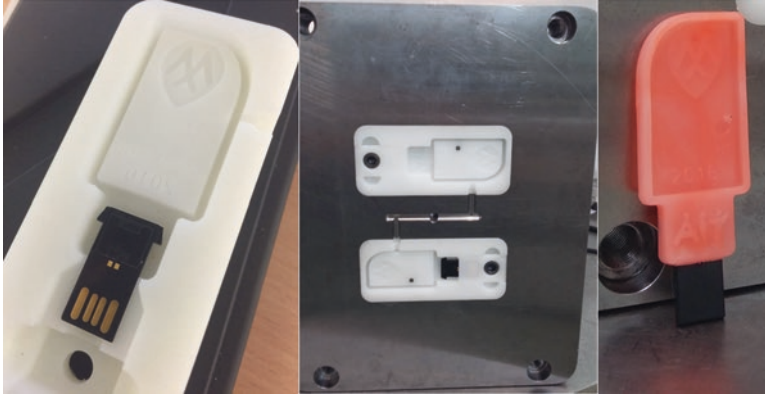
Fig. 4.4 Resin-based rapid tooling was used to produce USB keys from design to production in 3 days which represented 24 person-hours. (Left) the USB component loaded into the printed insert; (middle) inserts placed in tool; (right) moulded USB key
