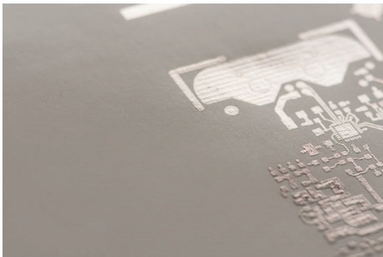
Fig. 5.2 Silver tracks deposited using material jetting
