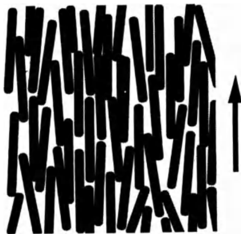
FIGURE 2.21 Nematic structure with the director indicated by an arrow. (Gedde, U.W., Polymer Physics , Chapman & Hall, 1995, p. 112)
