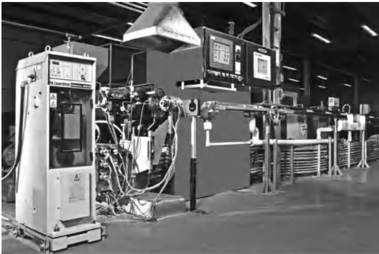
FIGURE 5.9 Extruder system with a cross-head. (Courtesy Davis-Standard, LLC).
