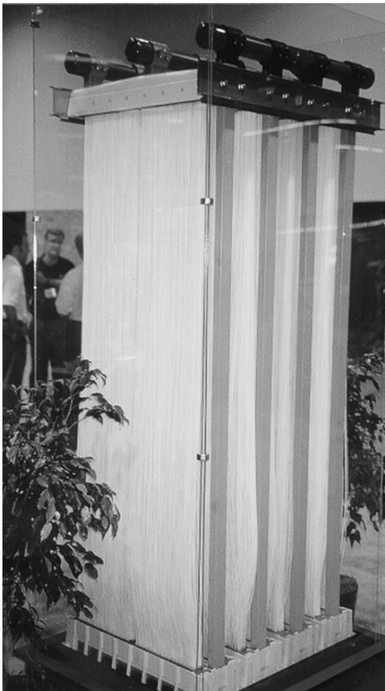
FIGURE 7.8 Spaghetti strand hollow tube membrane filter clarifier.
