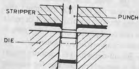
Fig. B7 Stripping jammed sheet from punch
