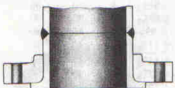
Cranelap Flange with Cranelap Stub End Butt-Welded to Pipe
