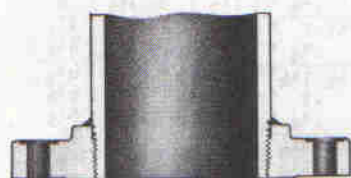
Screwed Flange Seal-Welded and Refaced
