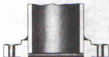
Type No. 1 Slip-On Welding Flange Welded Front and Back
