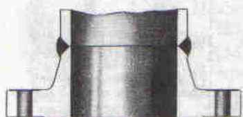
Welding Neck Flange Butt-Welded to Pipe
