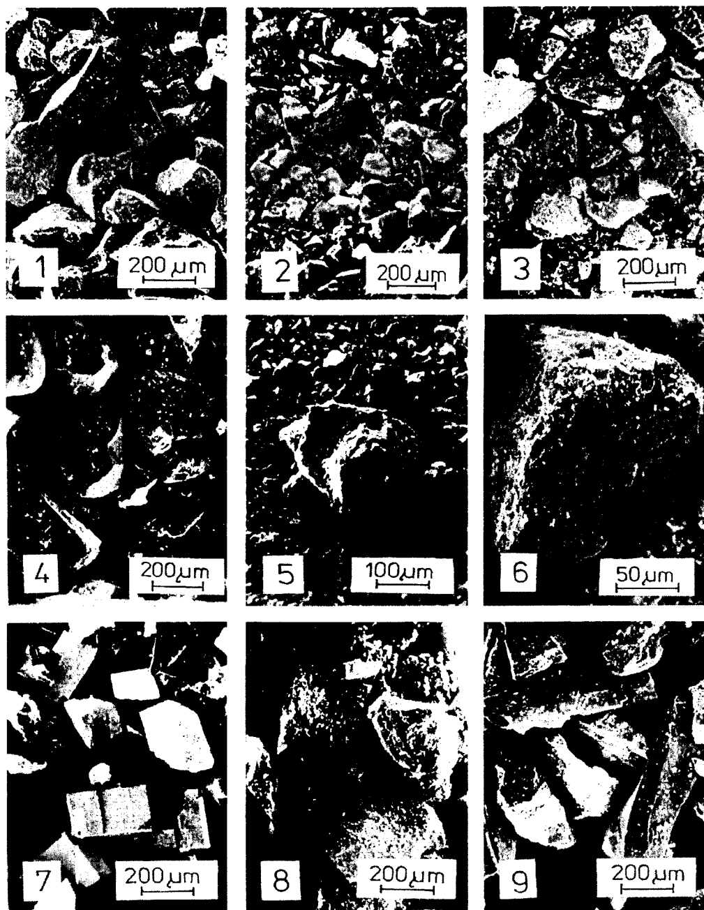
Fig. 3.3 Scanning electron micrographs of \text{CuFeS}_2 (1), \text{Cu}_{12}\text{Sb}_4\text{S}_{13} (2), \text{FeAsS} (3), \text{FeS}_2 (4), \text{Sb}_2\text{S}_3 (5), \text{HgS} (6), \text{PbS} (7), \text{Cu}_5\text{FeS}_4 (8), \text{ZnS} (9).
