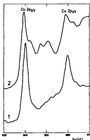
Fig. 3.22 \text{Cu}2p XPS spectrum of \text{CuFeS}_2 , mechanical activation: 1 – 0 min, 2 – 60 min [3.36].
