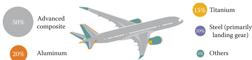
FIGURE 1.1 Use of various types of materials in Boeing 787. (From AERO-Boeing 787 from the Ground Up [Online], Available: http://www.boeing.com/commercial/aeromagazine/articles/qtr_4_06/article_04_2.html , 2017.)
