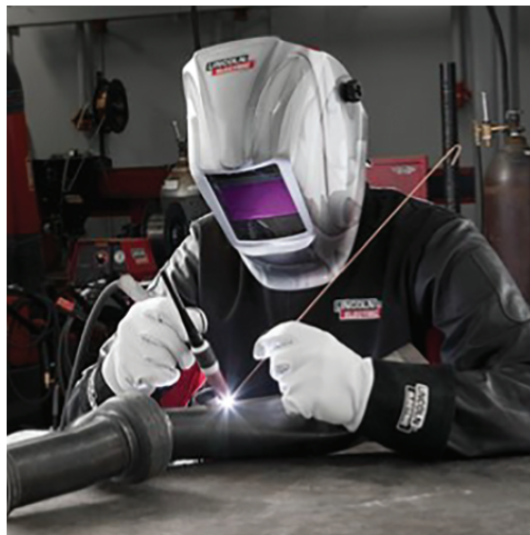
Figure 3.3.2 A GTAW welder, note the welding torch, and the filler wire in each hand.
