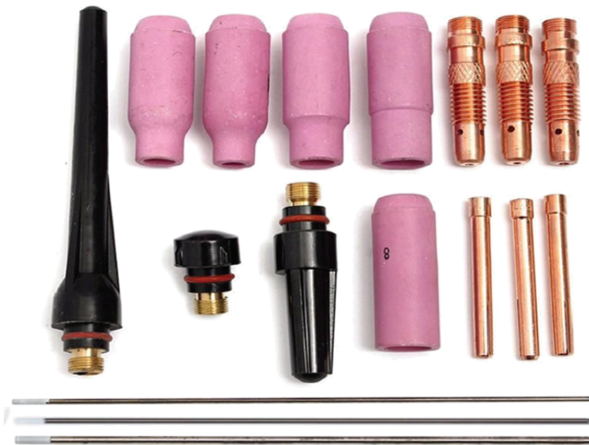
Figure 3.10.4 An assortment of manual welding GTAW torch components.
