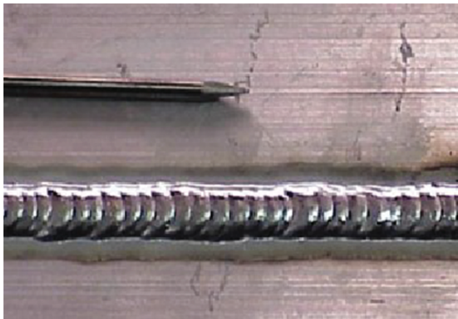
Figure 3.7.2.6 Weld profile as a result of reduced EN cycle.
