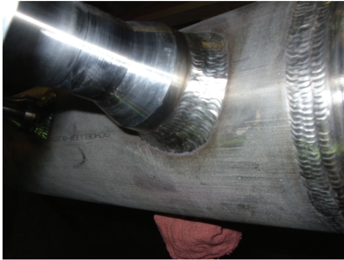
Figure 3.25.9.3.2 A nozzle is welded on a pipe header.
