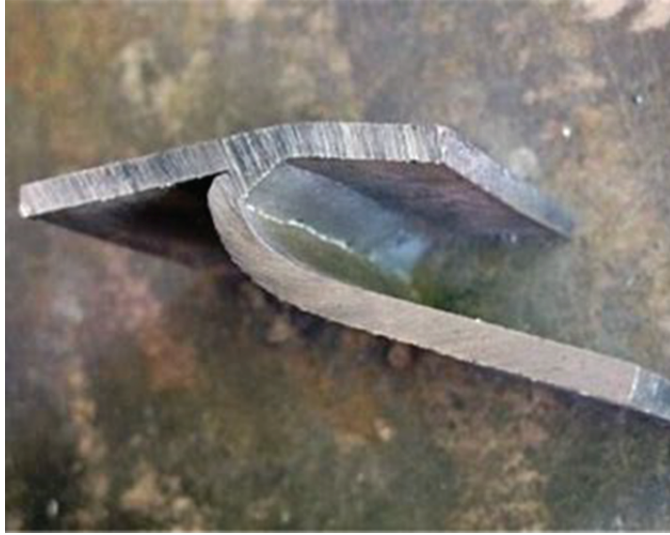
Figure 2.12.6 Aluminum fillet weld-bend testing.
