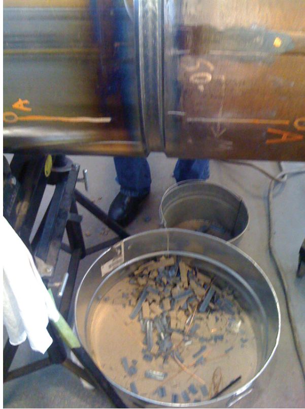
Figure 6.6.2 Shows the collected flux for cleaning and reusing.
