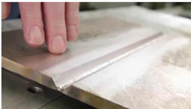
Figure 2.14 Nickel alloy plate being welded.
