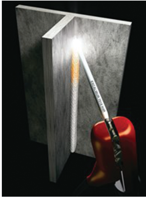
Figure 2.14.3 Nickel alloy welding (note the fillet weld in upward progression).
