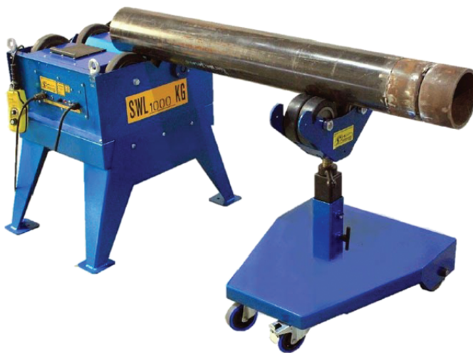
Figure 2.11.10 This rotator is similar to the one above except that the pipe end is placed on a motor driven set of rollers on one end, and the other end is on the set of idle rollers, which can be lowered or raised to align and level the weld joint.
