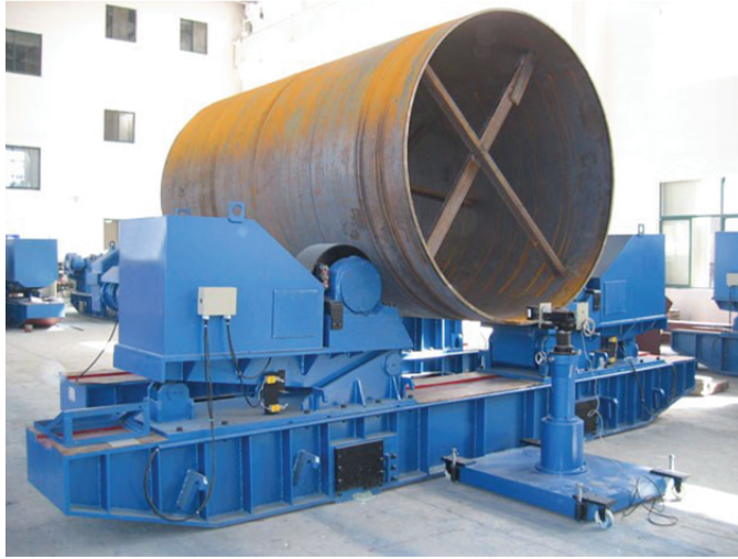
Figure 2.11.11 A heavy-duty rotator.
