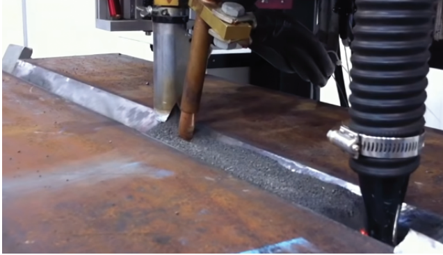
Figure 6.3.2 Shows the submerged arc welding of a plate.
